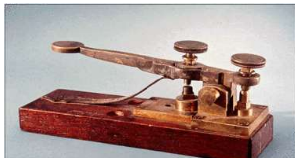
The telegraph machine works by sending a series of electrical signals through a wire, which are heard as long as short beeps. These beeps are a code, called Morse Code.
